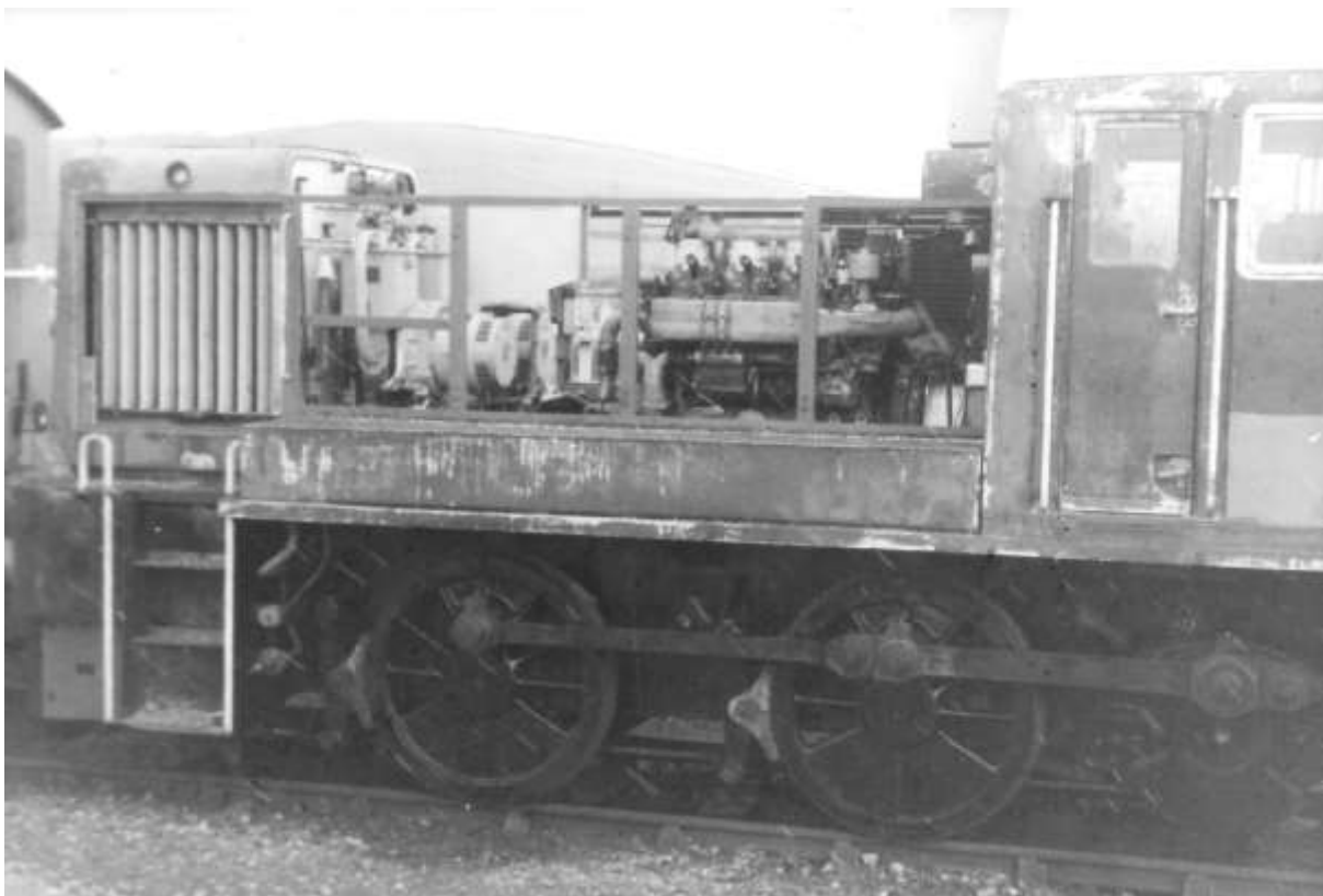
The engine has been rebuilt but is awaiting a turbocharger circa 1983
