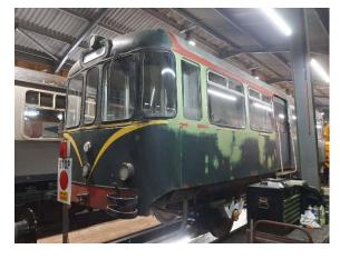
In this view, primer paint has been applied to the first section of repairs. Green anti-corrosive primer is applied to the bare steel and previously painted aluminium panels, red etch primer to the bare aluminium areas.
