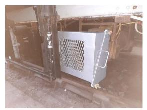
The repaired heater filter box seen in the last update has now been painted and refitted.
