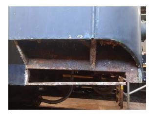
The droplight windows in each corner were all stuck in the open position, this has allowed rainwater into the vehicle and contributed to the damage to the floor and body frame. The scissors and spring mechanism has been repaired and now the droplights work correctly for the first time in many years! To access the mechanism the interior Formica panels and external valence panels had to be removed. As expected, this revealed further corrosion.
