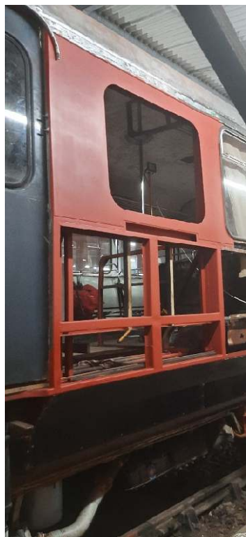
Frame repairs complete and primer painted.
