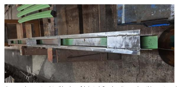
A new replacement waist rail has been fabricated. On a long item such as this, great care is required during welding as it is very easy to distort the assembly. Thanks to the skill and patience of Martin Luffman, the new rail turned out perfectly.
