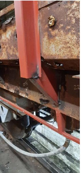
The new waist rail has now been welded in position, along with a new vertical body pillar.
