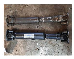
The original Cardan shaft was excessively worn in both universal joints and the sliding section.
