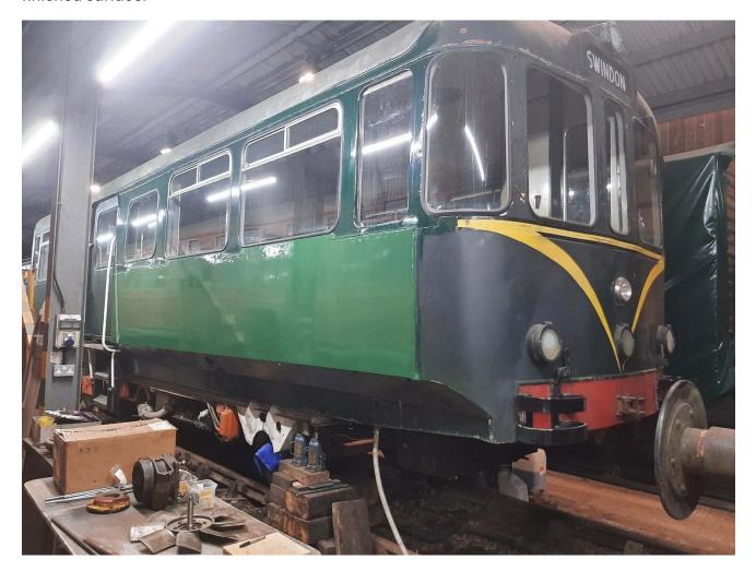
In addition to the panel repairs, here you can also see evidence of the other work being carried out, on the bench at the front are the radiator cooling fan and an axle bearing housing. The corner of the railbus nearest the camera has been raised on jacks to allow the axle bearing to be inspected, and on the other side are the containers which the engine coolant has been drained into.
