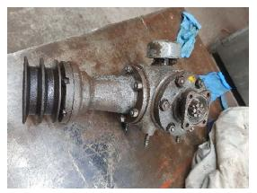
The right-angle drive unit has had new oil seals fitted on both input and output shafts.
