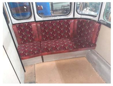
Retrimming is almost complete on the bay window seats at each end. Much of the original wooden framework for these had rotted away so there is a process of fit, remove and adjust then refit to get them just right.
