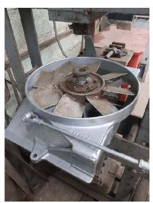
The fan housing has been shot-blasted and repainted, and the cooling fan reassembled with new bearings and seals.
