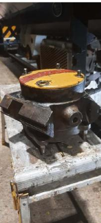
The axle bearings have all been inspected. This involves lifting the Railbus with hydraulic jacks and removing the suspension Chevron springs and axle bearing housing. The old grease is then removed, and the bearing carefully cleaned for a thorough visual inspection.
