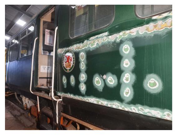
The outer panel refitted following last winter's body frame repairs has had all the rivet heads filled to create a smooth surface and has received several base coats of paint. The final gloss paint will be applied when the weather is more suitable and the mechanical works for this winter are completed, to reduce the risk of damaging the finished surface.
